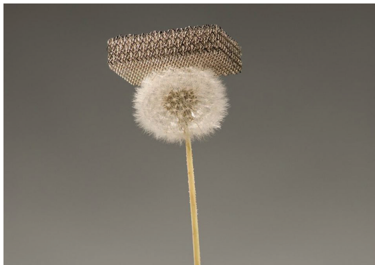
Figure 3: An example of the lightness of the Boeing composite
